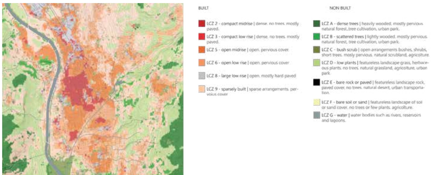
Figure 2. Local Climate Zones map resulted from mapping the classification of LCZs. The result consists on typological areas based on the combination of surface structure, cover and human activity. The map was obtained with the method described in Bechtel et al. (2015) and shows the 13 LCZs present in Trento.
